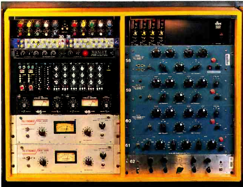
Detail of part of SSL I's outboard rack located behind SL-8000 G-series console. The impressive collection of new and vintage outboard equipment includes Pultec equalisers and Fairchild compressor-limiters
