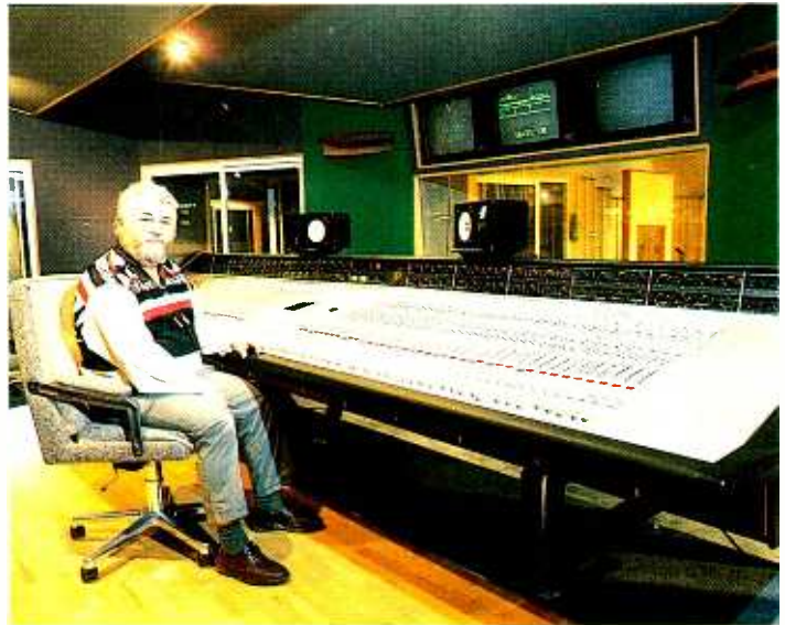
▲ Jerry Boys and Livingston's new 72-channel SL 4000 G Series console, fitted with the Ultimation dual automation system
