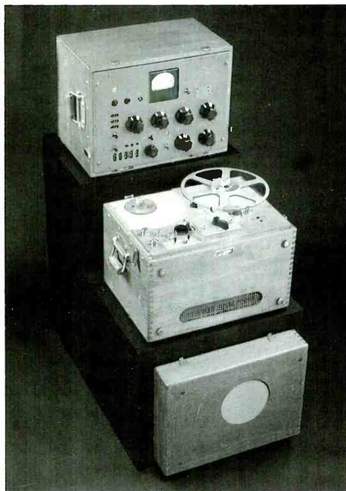
1951 — the model 27. The box behind the recorder is a 4-input mixer including record/reproduce electronics
