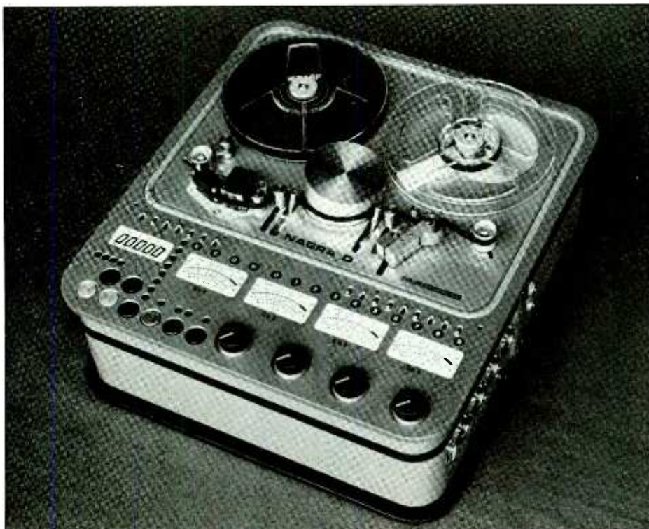
Nagra-D digital recorder—open reel with rotary heads
