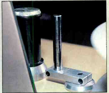
Fig 1 & 2: Before and after shots of a guide showing deposit from back coating
