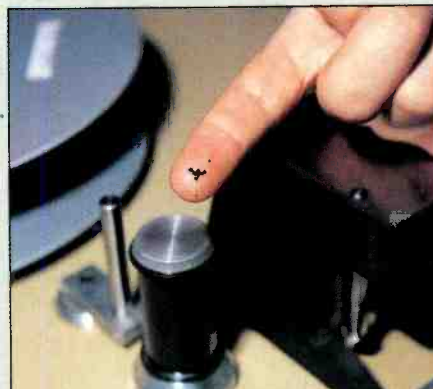
Fig 3: Scraped from the guide, the deposit is hard and shiny
