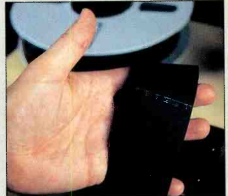
Fig 4: Damage to the back coat caused when guide deposit bonded tape to guide
