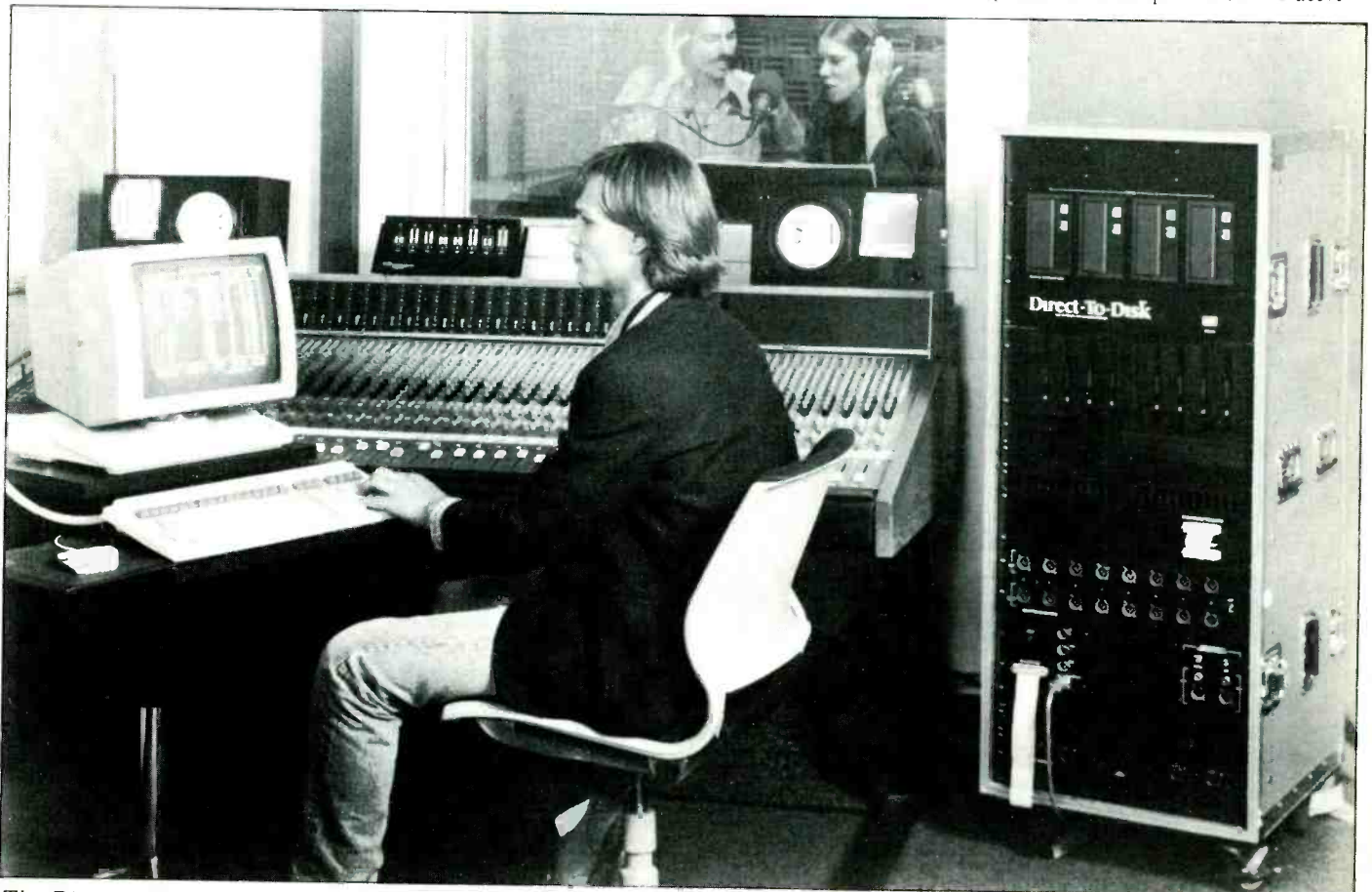
The Direct-to-Disk system in operation on a vocal session
