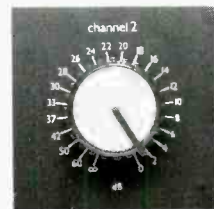
The V800 features stepped input attenuators
