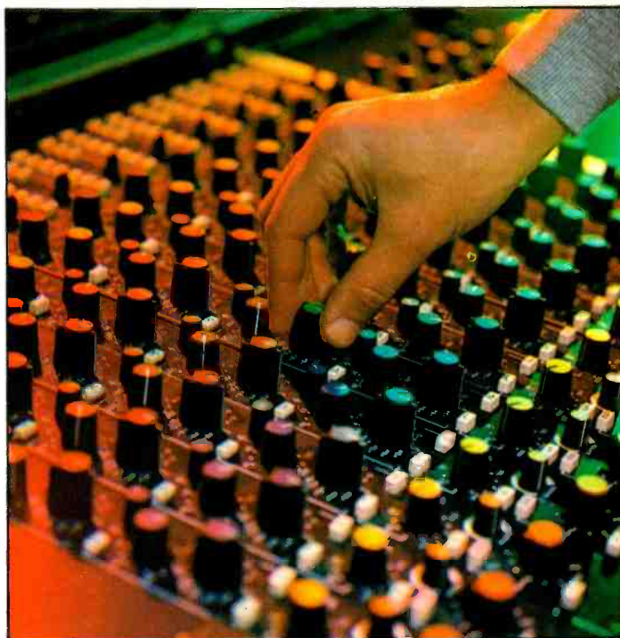
Fig 5: Adequate operating space reduces the likelihood of inadvertently moving other control knobs
