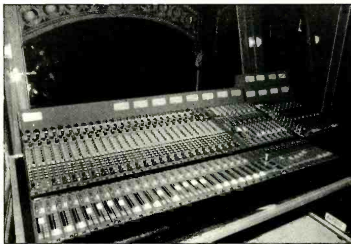
Midas TR System console, sub-console to the right
