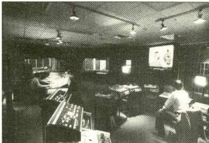
The dubbing mixer (left) has a good view of the main projection screen and the two commentary studios, while his assistant drives the 'mini-mixer' effects console.
