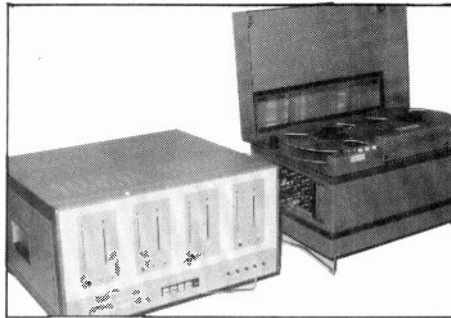
Soundstream digital 4-track recorder using electronics package and standard instrumentation recorder.
