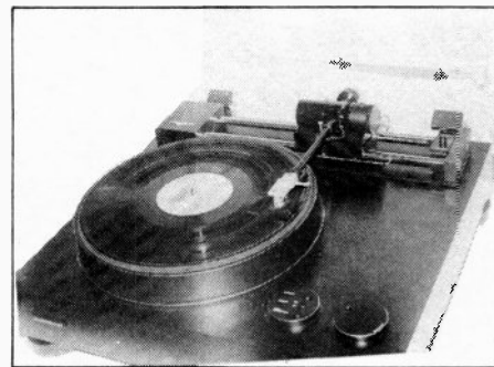
Pioneer turntable system with hanging rotor motor and linear motor drive tangential tracking tone arm
