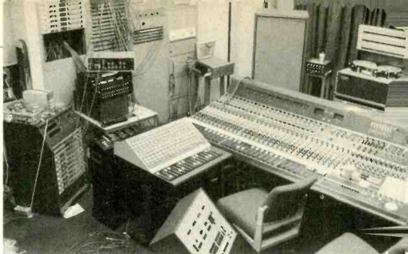
BBC Maida Vale Studio 6 'arranged' for the Genesis mixdown. Note Lyrec 24-track with remote controller by Neve console, BBC racked Dolby A units, and central equipment 'stack' comprising (top to bottom) Calrec Soundfield decoder, Eventide Harmonizer, Technics equaliser and BBC Matrix-HJ encoder.
