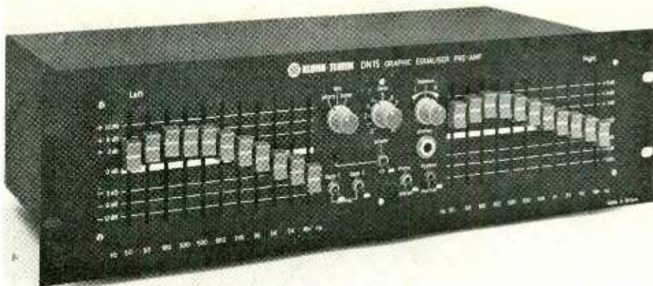
Klark Teknik DN15 stereo graphic equaliser incorporates a low level pre-amp
