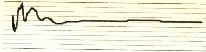
FIG. 2 Frequency drift of 20 Hz on setting frequency. 2 Hz per vertical calibration. Paper speed: 0.3 mm/s.
