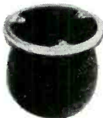
4021 OMNIDIRECTIONAL Moving coil 40 Hz - 12 kHz Impedance: 30 \Omega Output: -80 dB ref IV/dyne/cm 2
