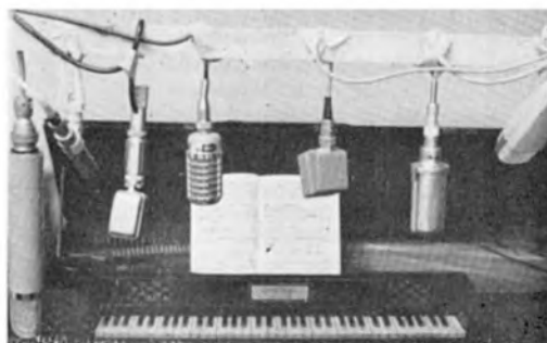
Fig. 6 The five microphones under examination, a Reslo , and the author's capacitor design, suspended above a Mozart piano.
