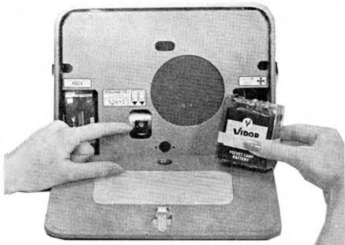
Showing the speed change button (left) and battery compartments.
