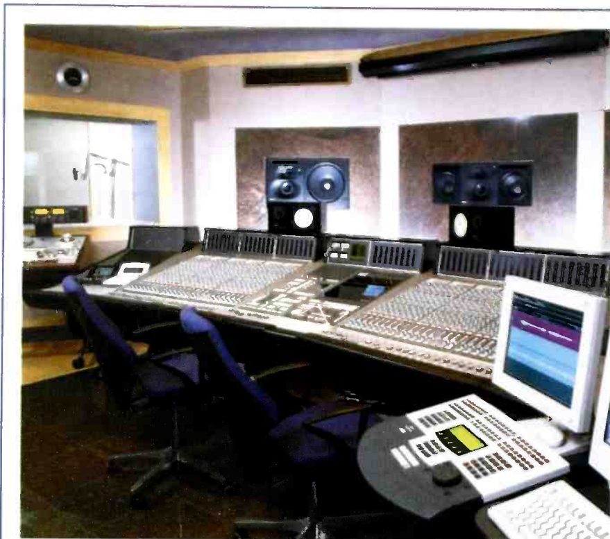
Brazil: Sao Paulo's music recording and DVD authoring facility Mosh Studios has installed a 48-track Fairlight Merlin recorder and 96-input SSL Axiom MT console for a new 5.1 mixing suite, designed by Jeff Sorbes. Since opening earlier this year, the suite has hosted DVD music video projects for the Universal, BMG, Warner Music Group, and Sony Music Entertainment record labels. Owner Oswaldo Malagutti Jr commented, 'In Brazil, the name Fairlight has a very good reputation. It inspires trust in the minds of producers and other clients... I knew that a Fairlight system would bring in business and pay for itself over time.'
