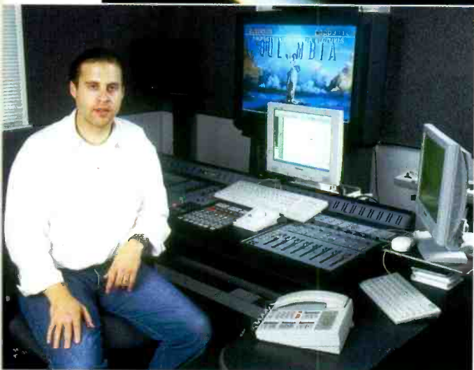
Steve Ticknor, FX editor and temp dub mixer in one of Sony Pictures' mix-to-picture suites. The room features a 32-channel /4-layer Digidesign Pro Control mixing system, linked to a fully loaded Pro Tools digital audio workstation with three 8:8:8 converters for 24-channel I-O. An Otari picmix handles multichannel monitoring and loudspeaker assignment, with PEC-DIR control switching for two Sony DADR-5000 digital dubbers
