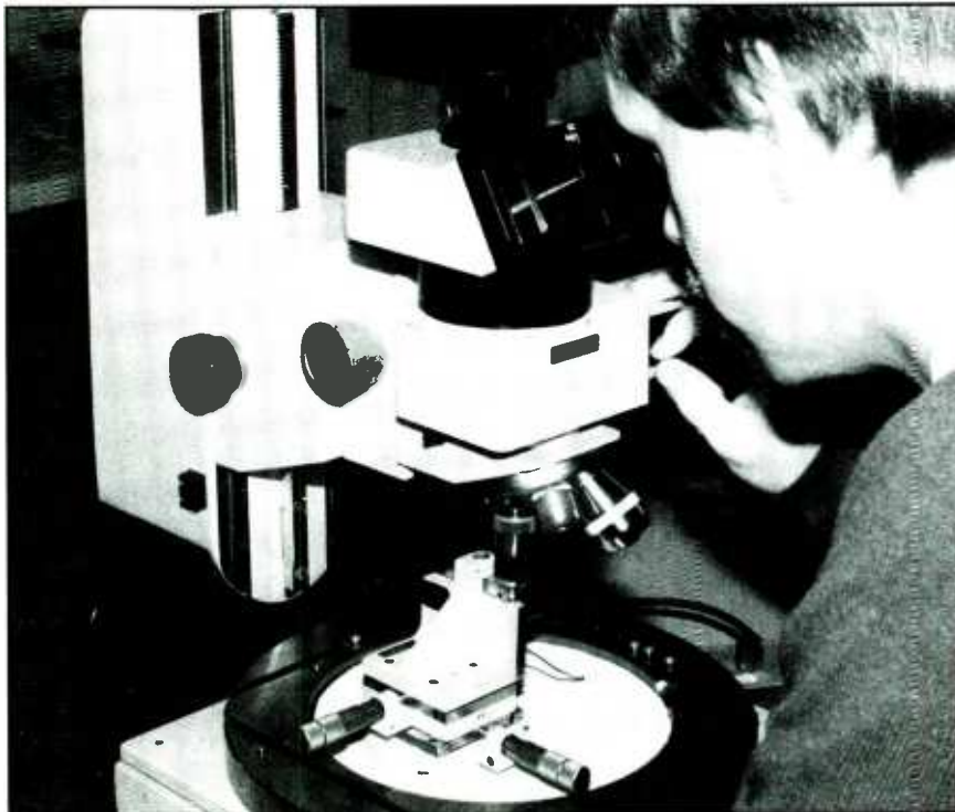
Individual heads are inspected for gap, lamination and ferrite material condition, as well as surface finish, all fully documented.
