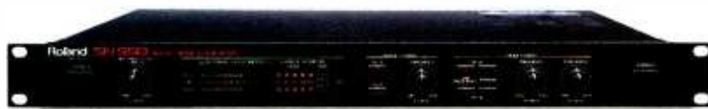
16-bit linear A/Ds and 18-bit D/As with 48kHz sampling frequency gives the SN-550 Noise Eliminator exceptional dynamic range and sound quality.
