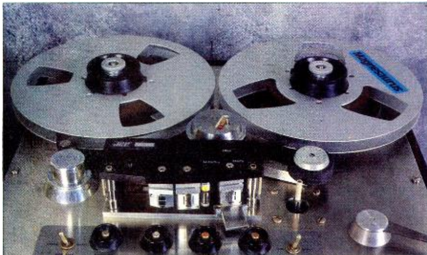
Improvements to the 351 include a replacement head nest (custom-modified Sony MCI), custom-made heads, rebuilt motors and a custom flywheel.
