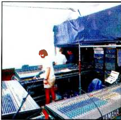
House engineer Gary Fox used Yamaha PM3000 consoles with signal processors from Yamaha, Lexicon, dbx and BSS.
