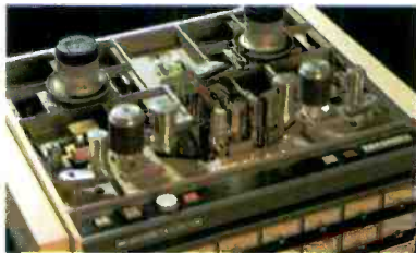
Otari isn't in the toy business. The MX-80 and MTR-90 sport 2" thick cast alloy deck plates, heavy duty swing arms, and motor shafts designed to handle the exceptional acceleration characteristics of these machines.
