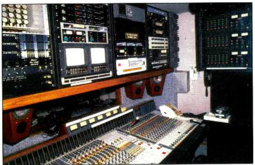
Figure 3. Interior shot of the audio control section of NEP's remote truck, which was crewed by Dick Clark Productions. Stereo audio feeds from the Fanta and Westwood One remote audio units were monitored here, along with a reference mix from the live P.A. mixing equipment.
