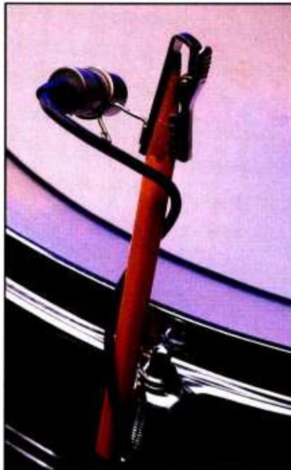
Try experimenting with different mics and positions for unusual sounds. For example, try a lavalier mic attached to a pencil, which is then taped to the snare drum. Does a No. 2 lead sound better than a No. 3? Try it and see what happens.
