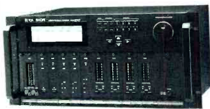
The TOA Saori is a modular processing system for sound-reinforcement applications.
