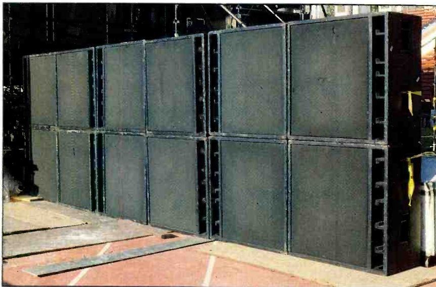
Photo 2. Group of eight 2x18 Clair custom subwoofer enclosures, positioned at ground level.
