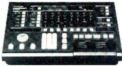
Tascam showed a final software version of the MIDIiZER, a 2-machine transport synchronizer.
