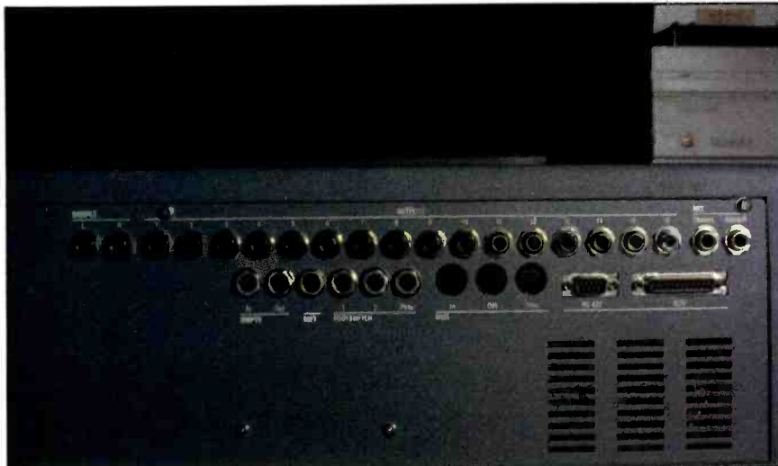
Photo 3. Back panel of the Emulator III showing SCSI, RS-422, MIDI and SMPTE interfaces.
