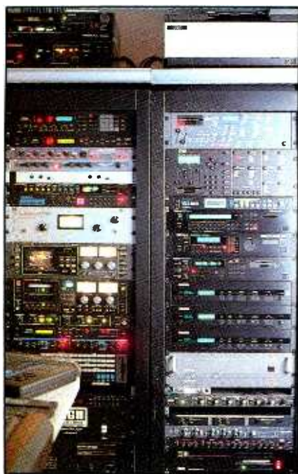
Photo 2. Two racks of outboard equipment, including rack-mount sound sources and various signal processors.
