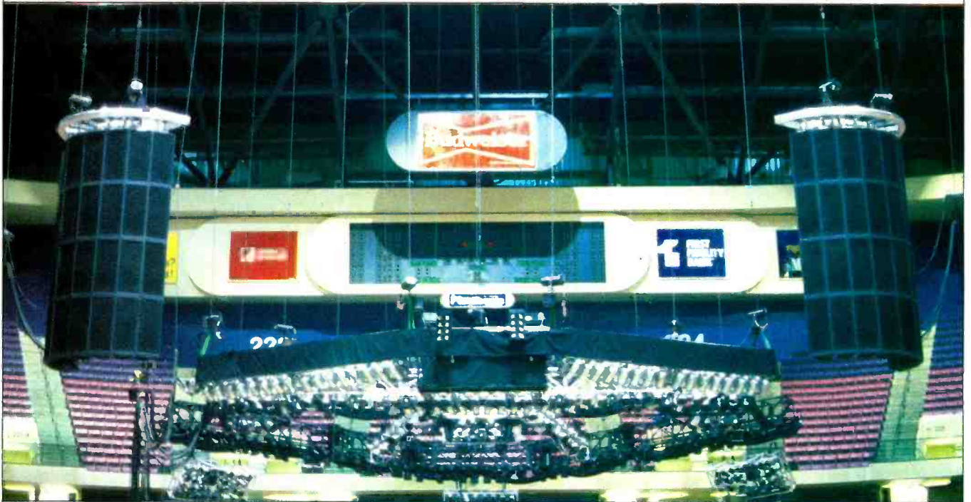
Figure 9. The Prism arrays shown in an arena setting. Note that the array appears vertical when viewed from nearly any angle.
