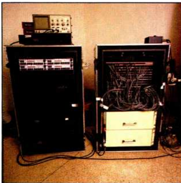
Closeup of racks No. 2 and 4, containing a patchbay, monitor amplifiers and Lynx TimeLine synchronizers.
