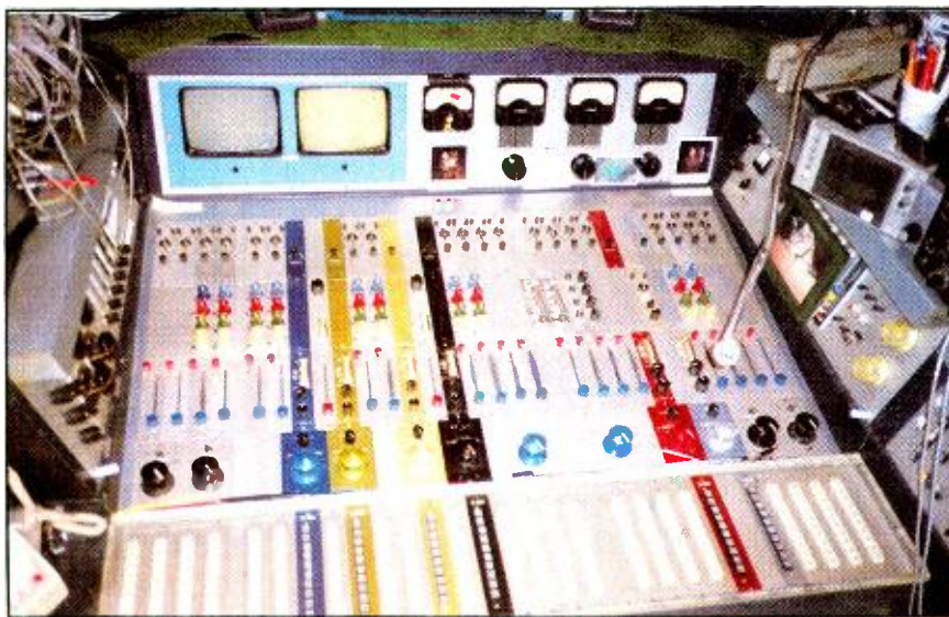
Photo 1. Close-up of the old console, showing assignment push-buttons under the armrest. Notice the rotary submasters and masters immediately above the arm rest. Next are the 22 vertical faders with 10 subfader groups above. The equalizers for the vertical faders are at the top.
