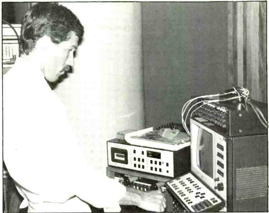
Figure 5. Richard Craig, B&K field applications engineer, observes the acoustical response of the sound system in the room. Meyer CP-10 parametric equalizer is used for EQ adjustments.
