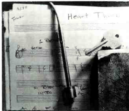
Figure 16. Mic element used for saxophone pickup rests against sheet music; key shown for scale.
