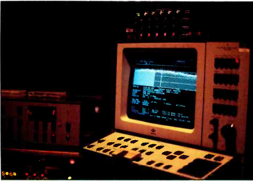
Figure 4. The Bruel & Kjaer model 2032 dual-channel FFT signal analyzer.
