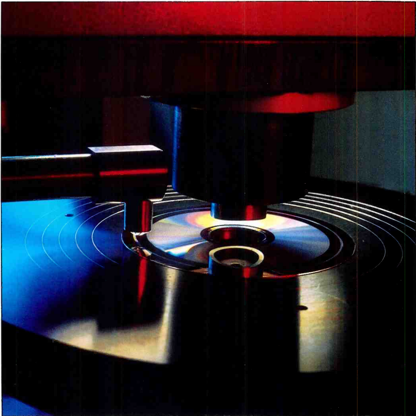
Removing a recently manufactured disc from the stamper.
