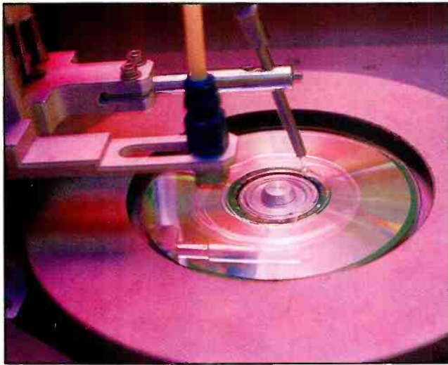
Applying the lacquer on a metallized disc.
