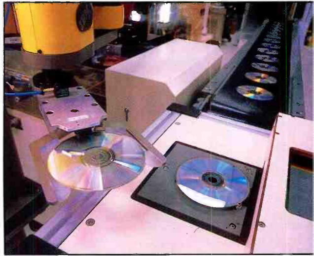
Robot arm transferring the lacquered disc to the printer.
