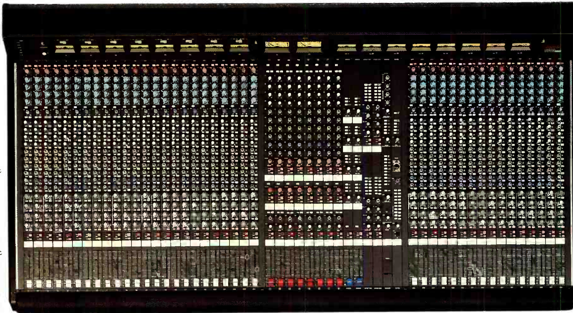
WR-S840 Configured as a 40 x 18 Stage Monitor Console.
