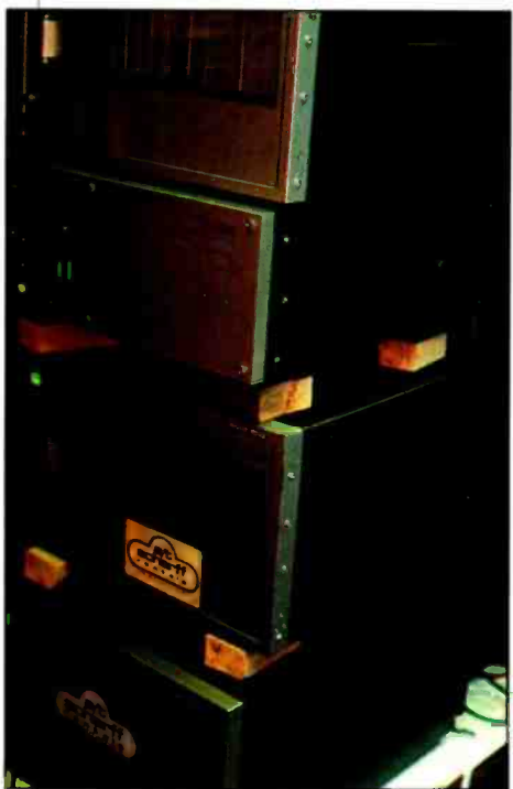
Stacked in the rear of Caedmon Records' control room (top to bottom): Sony PCM-1610, 1630 and a second 1610 digital audio processor, plus the electronics cabinet for the Sony DAE-1100 digital editing system.
