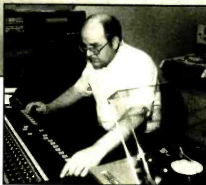
Recording and production equipment available at the Association of Baptists for World Evangelism's Media Center includes a Yamaha RM2408 console and various Otari MX-5050 and MTR-10 multitrack and mastering transports. Pictured here in the central control room area is Bob Henry of the ABWE production staff.
