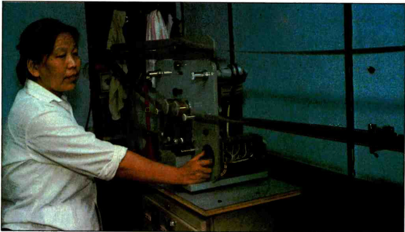
A 35mm looping recorder at the Beijing Film Studio used in Foley and dialogue replacement.
