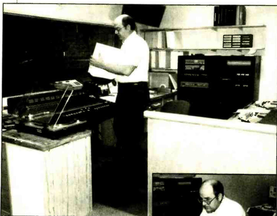
Recording and production equipment available at the Association of Baptists for World Evangelism's Media Center includes a Yamaha RM2408 console and various Otari MX-5050 and MTR-10 multitrack and mastering transports. Pictured here in the central control room area is Bob Henry of the ABWE production staff.
