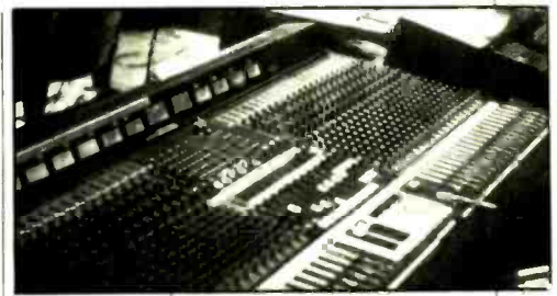
Figure 4. The house mixing position featured a pair of Yamaha PM-3000 consoles and a Soundcraft 200-B submixer.
