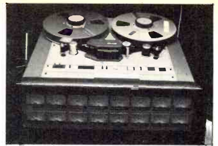
Left: Outboard units include a Roland DM-3000 delay, Ibanez UIE-405 and HD-100 effects, MXR 01 reverb and DOD R830 graphic; Below: Tascam Model 15 mixer; Right: Tascam MS-16 16-track.
