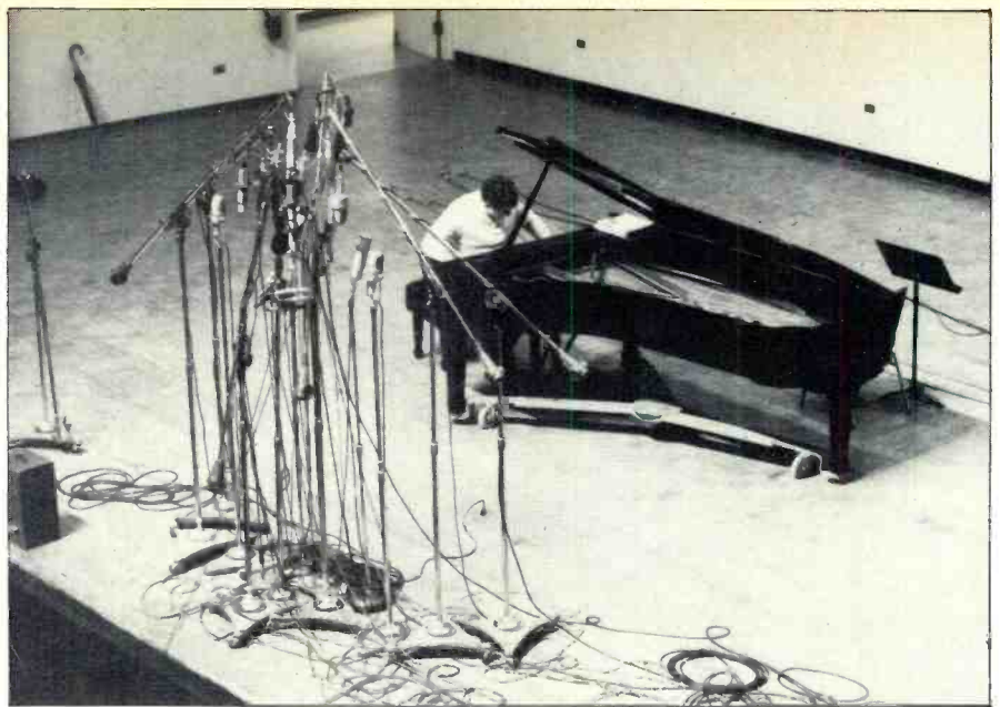
Stage area of Clapp Recital Hall during May, 1985, evaluation sessions, showing microphone layout and distance to grand piano.
