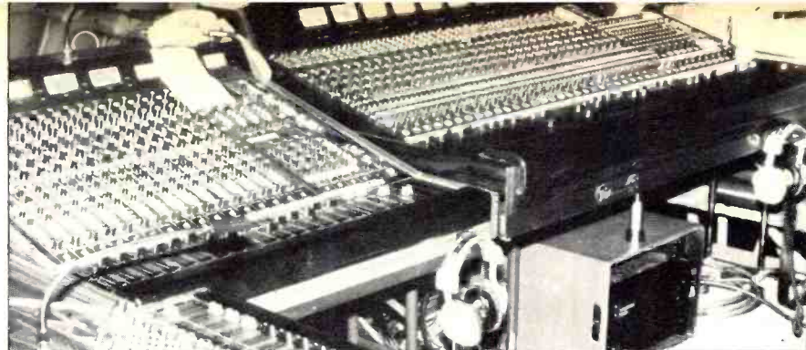
Figure 15: Audio Techniques relies on Yamaha mixing consoles. Shown here: a PM-2000-32, an M1516, and an M-508.
