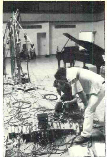
Peter Nothnagle (left) and Bill Bradley with collection of tube-mike power supplies and microphone connect cabling.
