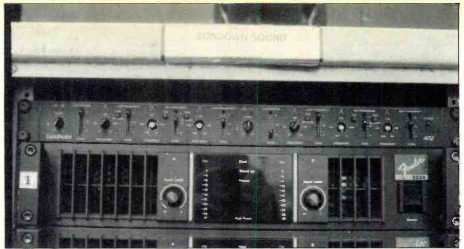
Figure 5: A compact electronic crossover from Sundholm Electronics is included with each power amplifier rack. Crossover points are 200 Hz and 1.6 kHz.
