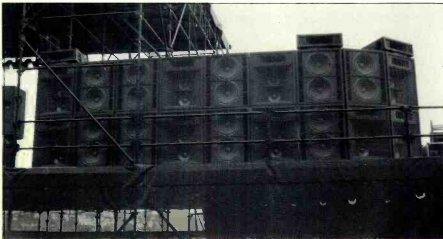
Figure 12: When a group of SDS enclosures are stacked together, a tight, compact array is formed. Here, one side of the 36-cabinet system supplied to the 1985 Del Mar Fair in Southern California is shown.
