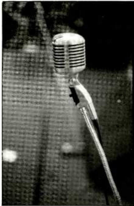
Figure 8: The Shure SM-55, an old standard, is favored for vocals by band members, with one important difference: the microphone has had an SM-57 capsule installed at the Shure factory.
