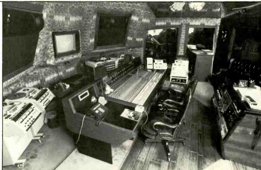
Main control room at Omega Audio, designed for 24/46-track recording, video sweetening, and mixdown. Equipment includes an AMEK 2500 console, and Otari MTR-90 24- and MTR-10 two-track machines.
