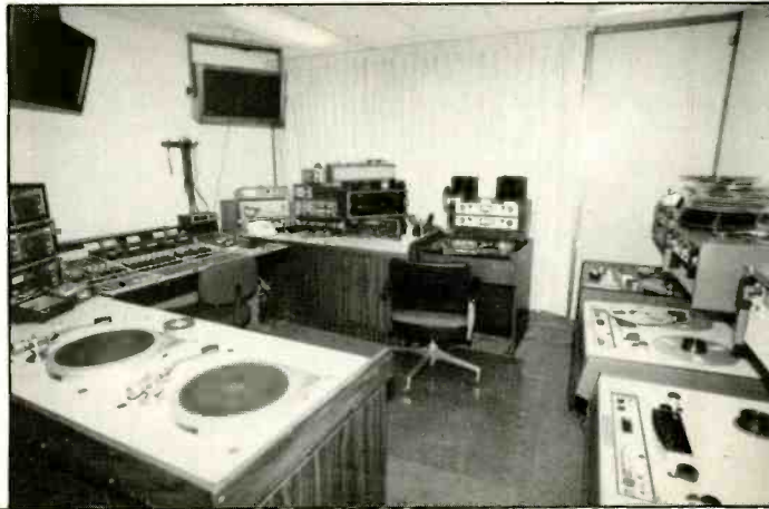
Studios D (left) and C feature identical McCurdy production consoles equipped with 24 stereo input channels. Available tape machines include MCI JH-110 two- and four-tracks, Scully 280 and SP14 two-tracks, and ITC Series 99 cartridge transports. Turntables are Russco and direct-drive Technics.
