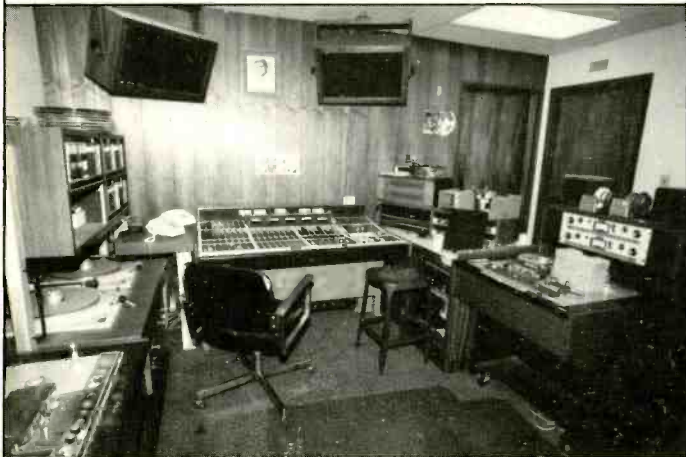
Studios D (left) and C feature identical McCurdy production consoles equipped with 24 stereo input channels. Available tape machines include MCI JH-110 two- and four-tracks, Scully 280 and SP14 two-tracks, and ITC Series 99 cartridge transports. Turntables are Russco and direct-drive Technics.
