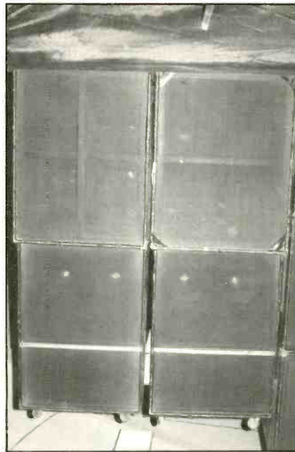
Figure 1: Two-box, four-way loudspeaker system set up on stage-level sound wings. Cabinets shown stacked vertically here are at the outer edge of the speaker stack, only a few feet from the wall.
