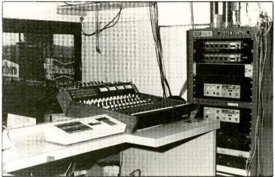
The Audio Control Area features an E-V Tapco Series II console. Signal processors include an Eventide Harmonizer and a UREI Model 539 LF rolloff filter.
