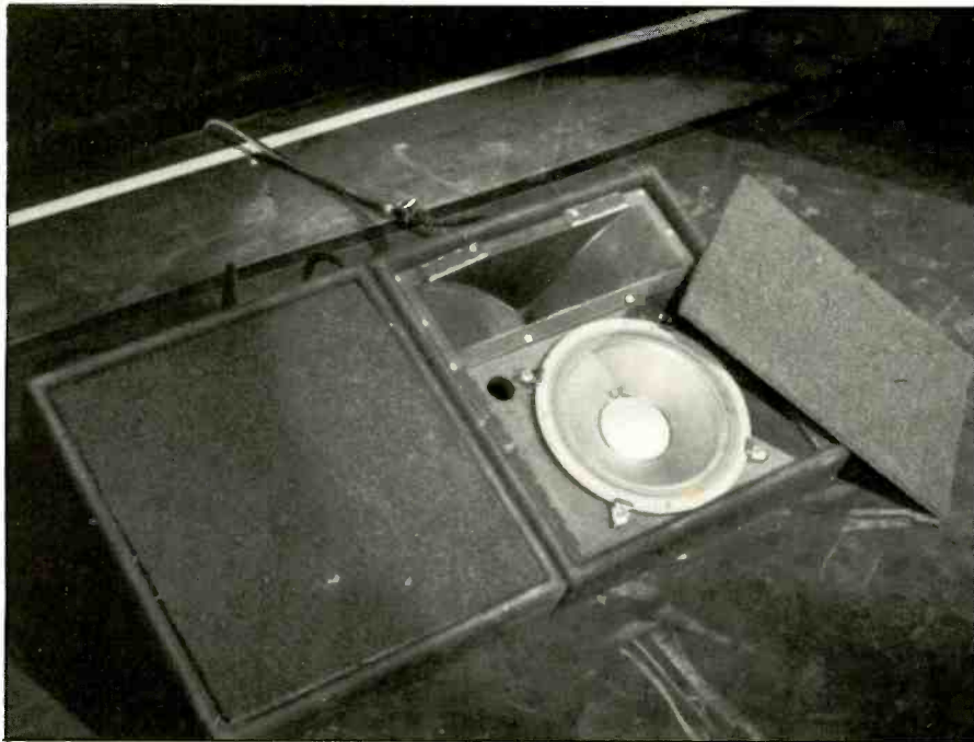
Figure 7: Low-profile floor slants were paired to give each performer an increased low-frequency presence.
