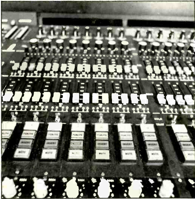
Close-up detail of the control surface switches, linear faders and control elements for a group of echo/foldback and channel insert/mute/enable modules (left), and an API Model 550A equalization module (right).
