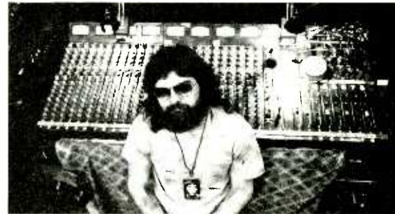
Monitor mixing engineer C.J. Patterson in front of the Midas 24-in/8-out monitor mixing console.
