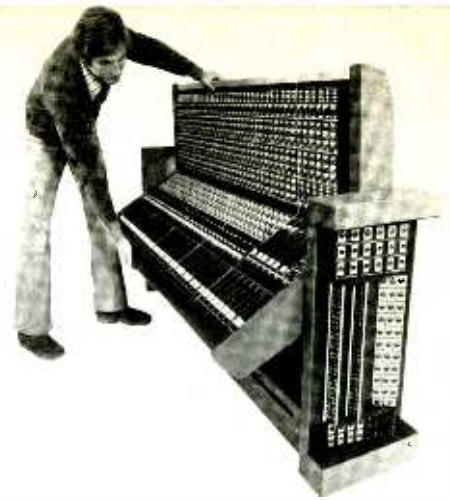
Figure 12: Clair Brothers' custom-built 32-in/6-out house mixing console. For ease of transport, the two sections are hinged along the center line, and fold together and down parallel with the sides of the board.
