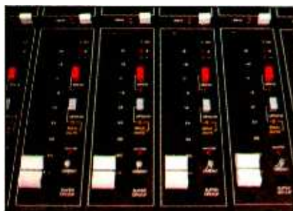
SuperGroup shows console group status at a glance, eliminating the need to scan each module.
