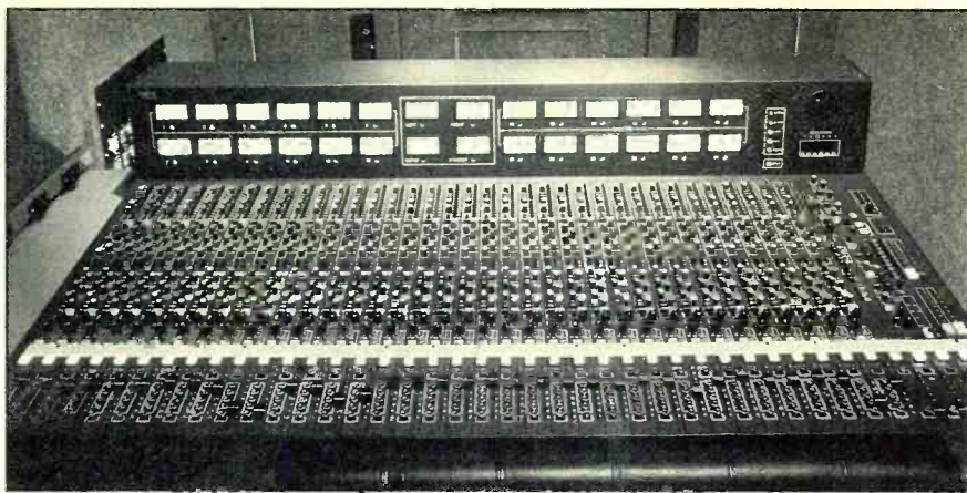
MCI JH-600 console fitted with 36 inputs, routing to 24 busses.
