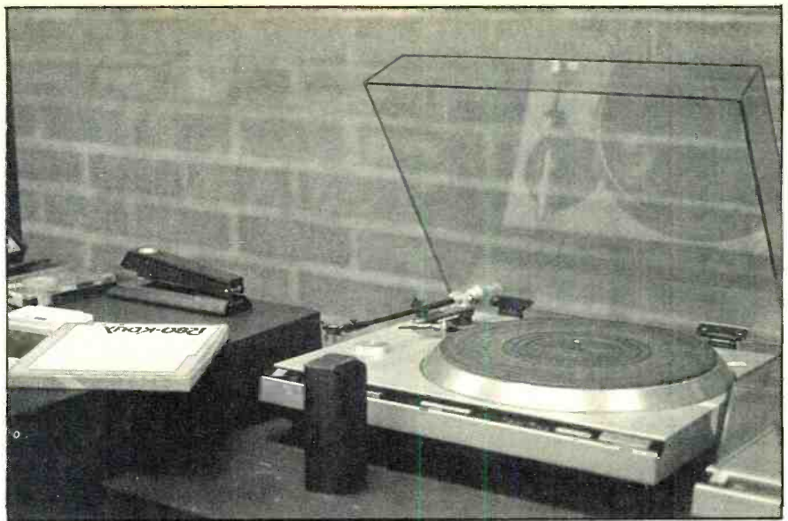
Technics SP10 MkII turntable and SME tone arm, mounted in isolation base
