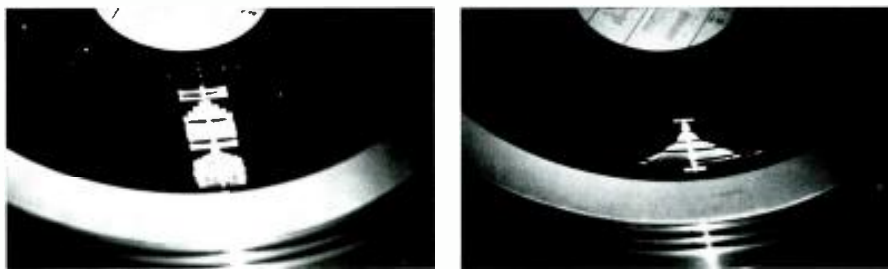
Left: Buchmann-Meyer light pattern on JVC Test Record (TRS-1000), no RIAA equalization, 5.0 cm/sec., all same level. Right: The RIAA playback curve below 1 kHz is depicted on this test record. The equalization required by the RIAA curve is applied gradually, hence, the light plot takes a "Christmas Tree" form.
