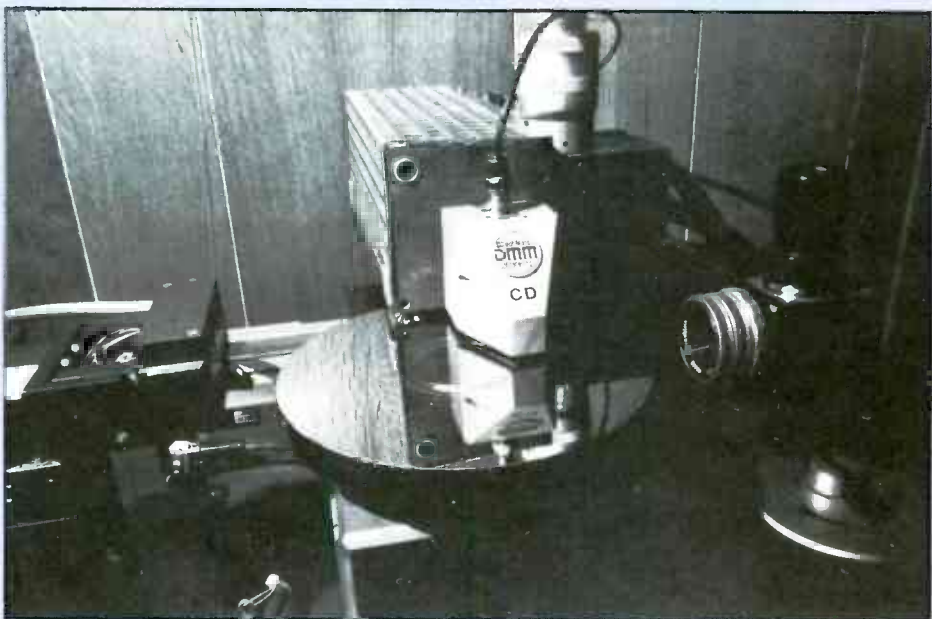
Prototype DMM-CD lathe. Above. Overall view of lathe, embossing head and carriage (master embossing recorder). The black tube (centre foreground) is the air supply to the bearings. Below. Detail of embossing head and copper master. To the left of the picture is the laser pickup for the depth control in its fully retracted position.
