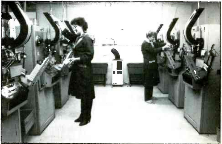
King 790 computer controlled cassette loading machinery
