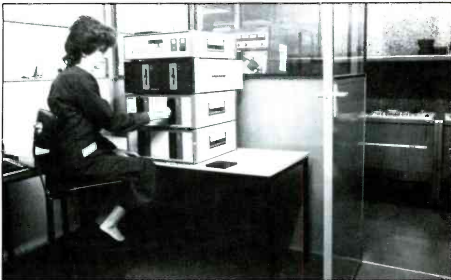
Floppy disk duplication. Computer cassette duplication bin and slaves in the background
