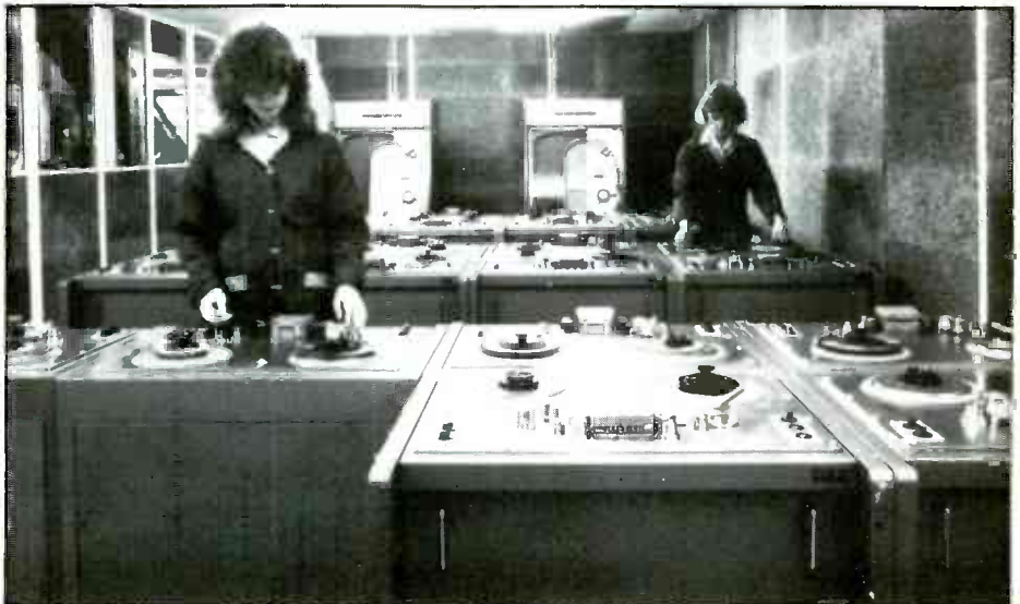
Main duplication area — general view of two jins and slaves
