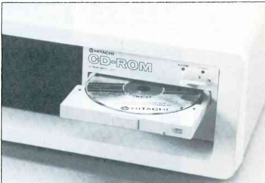
Hitachi's CDR-2500 CD-ROM built in to IBM XT
