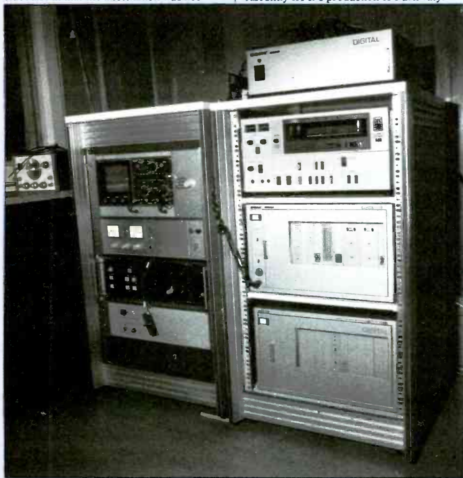
Sony equipment and prototype electronics for the DMM-CD
