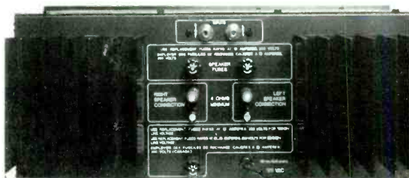
Spectro Acoustics 200SR: Close-up view of connection terminals on amp's rear panel.
