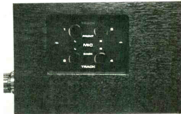
Dokorder 1140: Mic inputs are located on side surface of electronic section. (Phone jacks for front and rear channels are on opposite side.)
