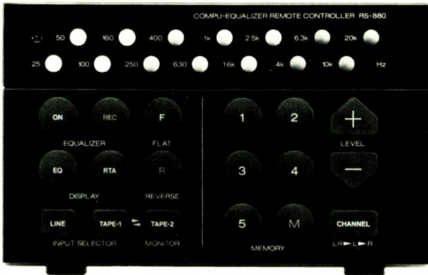
THE SE-88'S CONTROL MODULE DETACHES FROM THE FRONT PANEL FOR REMOTE OPERATION.
