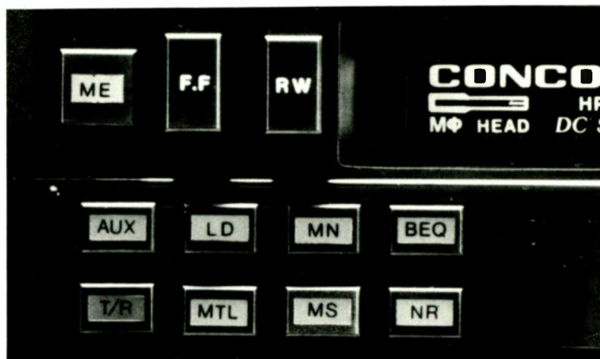
THE AUX BUTTON ON THE CONCORD HPL-550 CAN BE USED TO SWITCH IN AN EXTERNAL PROCESSOR.
