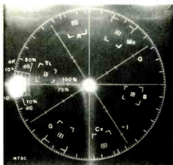
COLOR CONSISTENCY of the AVS-6200's recorder section (left) and TV tuner (right). In each case, the ideal would be for the cluster of dots toward the left edge of the grid to be a single dot at the intersection of the nine-o'clock axis with the circumference. The radial spread of the dots indicates chroma differential gain—a measure of how much color saturation (chroma level) varies with changes in scene brightness (luminance). The angular spread shows the chroma differential phase, which tells how much hue (chroma phase) shifts with changes in brightness. The VCR's performance is perfect, and the tuner's is excellent, with most of the error concentrated at the highest brightness level.
