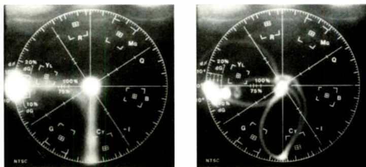
COLOR CONSISTENCY of the VH-5845XQ's recorder section (left) and for its TV tuner (right). In each case, the ideal would be for the cluster of dots toward the left edge of the grid to be a single dot at the intersection of the nine-o'clock axis with the circumference. The radial spread of the dots indicates chroma differential gain—a measure of how much chroma level (color saturation) varies with changes in scene brightness (luminance). The angular spread shows the chroma differential phase, which tells how much chroma phase (hue) shifts with changes in brightness. The VCR's performance is, again, perfect, and the tuner's is excellent, with nearly all of the error concentrated at the highest brightness level.
