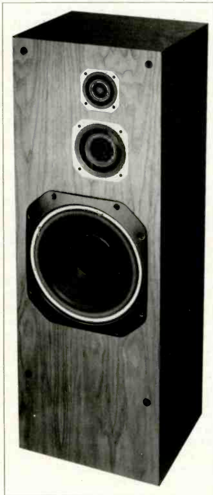
Magnavox SD-2570 loudspeaker system, in particleboard enclosure with walnut veneer finish. Dimensions: 14½ by 41 inches (front), 13½ inches deep. Price: $800 per pair. Warranty: "Unlimited," 12 months parts, three months labor. Manufacturer: Magnavox/N.A.P. Consumer Electronics Corp., P.O. Box 6950, Knoxville, Tenn. 37914.
