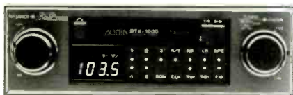
Clarion Audia DTX-1000 front end: Diversity reception gives a head start in the fight against multipath distortion.
