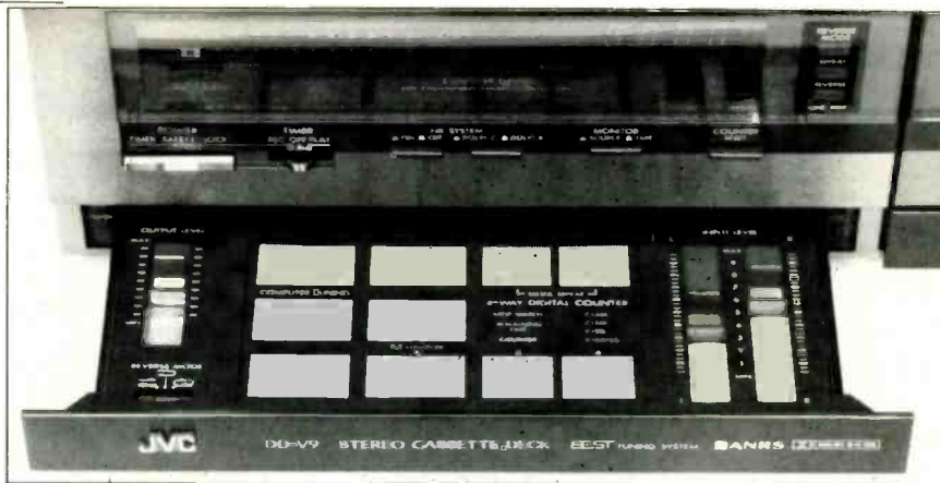
Most functions, except those relating to the tape transport, are controlled from this slide-out tray at the bottom of the front panel.
