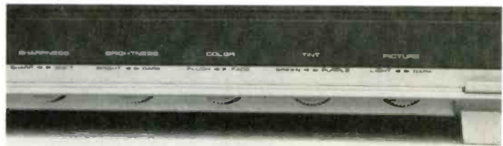
THE TVM-190'S CONTROLS are thumbwheels arrayed along the right end of the monitor's front panel, below the screen. They include adjustments for sharpness (detail), brightness, color saturation, tint, and "picture." The last is a combination control that affects both contrast and brightness. All except color and TINT have detents at their "standard" settings; these two must be adjusted by eye, since the TVM-190 has no automatic color-control or VIR circuitry to do the job for you.
