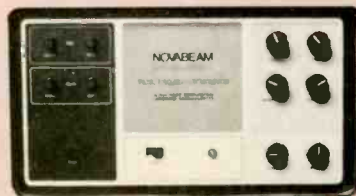
All controls are organized in one panel atop the projector. (Future production will move the controls to a hand-held wired remote.) The audio and video inputs and a front-firing speaker are located below the Novatron tubes.
