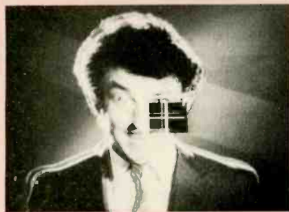
A built-in test-pattern generator makes convergence adjustments simple and precise. Horizontal and vertical controls for the red and blue images are rotated until they converge with a stationary green image, creating a single white cross.
