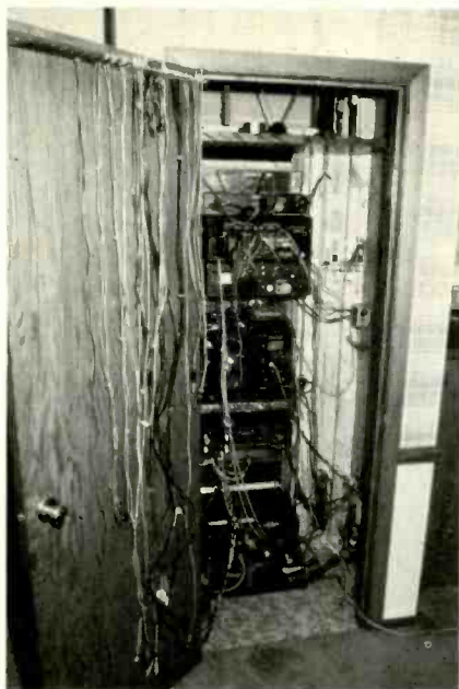
A door in the den opens to reveal the components' back panels. Cable racks on the door and a tool holder on the wall contribute to the setup's functionality.
