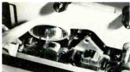
A dental mirror (left center) simplifies physical examination of often inaccessible tape heads for dirt and oxide buildup.
