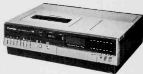
Both Beta and VHS VCRs look essentially the same on the outside, and, generally, they have the same features. The main difference is in recording time and tape path (see following pages). Shown are Panasonic's PV-1400 (above), a VHS machine, and Toshiba's V-8000 (below), a Beta deck.
