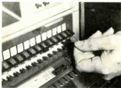
Translucent numbers are used for the sixteen tuners, twelve of which are assigned to the main screen. Channels may be in any order.
