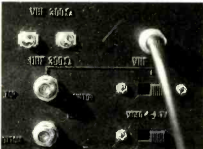
Back-panel switches and inputs let you monitor two VCRs simultaneously on the small screens.
