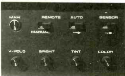
Controls for main screen, color-locking, and ambient light sensor are behind flip-down door.
