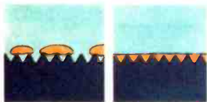
Artist's representation. Water-based record-cleaning solutions bead up on the grooves (left). Sound Life with super-wetting action deep-cleans grooves (right).
