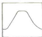
Distorted waveform response produced by conventional receiver.
