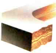
Low plastic base, particle board base is susceptible to vibration.
