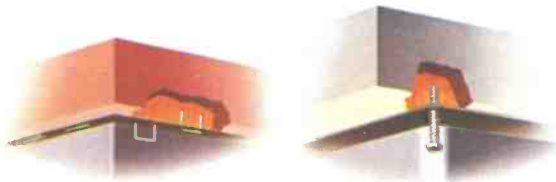
Common staples can work themselves loose, which is why Pioneer uses aluminum screws to mount the base plate to the base.
